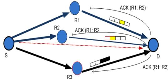
**Fig. 6** Frame combining at destination by scheduler.
