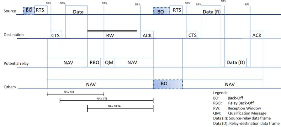
**Fig. 9** An illustration of RelaySpot's proactive mode.
