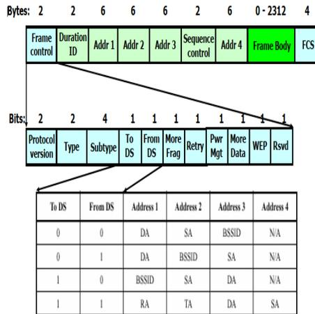
**Fig. 8** 802.11 frame structure used by RelaySpot.
