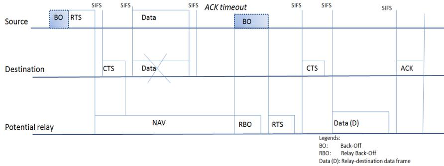
**Fig. 10** An illustration of RelaySpot's reactive mode.
